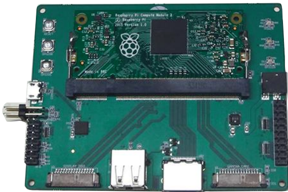
5. This Raspberry Pi Compute Module 3 is mounted in Gumstix Pi Compute Dev Board created using its Geppetto web-based design-to-order (D2O) system.
